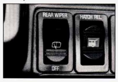
To release the hatch and unlock the doors from the inside of the vehicle, press the HATCH REL switch on the instrument panel. It is located on the driver's side of the steering column. The hatch will release with or without the key in the ignition.
